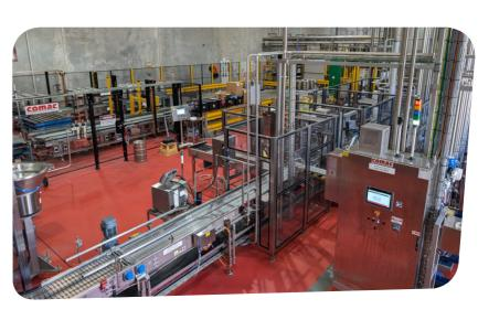
Coastal Electrics were engaged by TFG Group to disconnect and remove the redundant bottling and packing system at Lion Nathan's Perth facility, while maintaining the operational status of the plant. Coastal Electrics installed the power provisions for the new Keg Line before being engaged by COMAC to complete the electrical installation and commissioning of the new Keg Line and Boiler.
